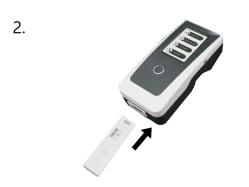
Scan the strip bar code, match corresponding standard curve data, and then test.
